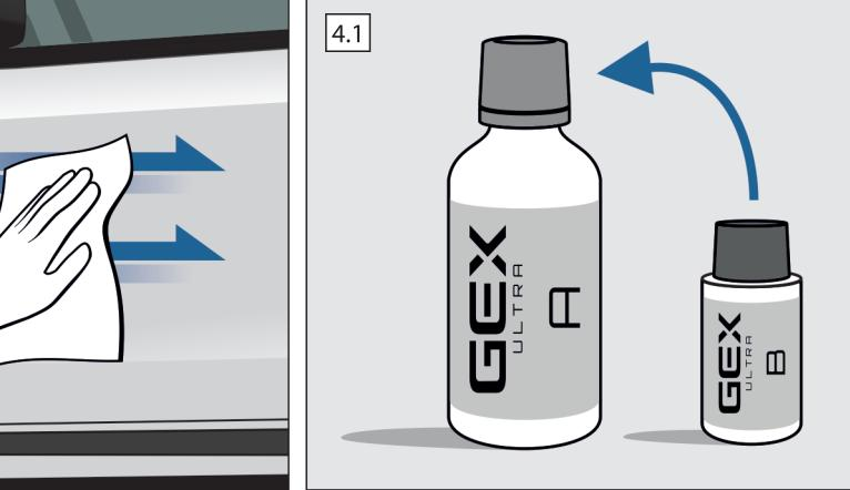
**Step 3.** Apply GEX Prep 200 ml from the kit on surfaces to be treated. Using the sprayer, apply the GEX Prep, spread it and polish with a piece of clean dry microfiber cloth from the kit. Apply step by step, treating the body elements one by one. Perform finish polishing of the surface with light straight movements (do not perform circular movements), without stroke marks remained.
