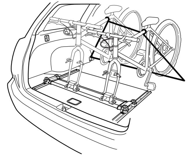
Be sure to fasten the Belt to the vehicle cargo hooks. It fastened the Belt to the hook of this Luggage Rail, the bicycle do not hold securely.
