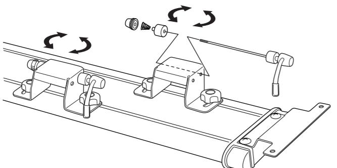
Mount the bicycle on the right side first. Adjust the position of the quick release and the angle of the fork mount bracket, for avoiding contact.
