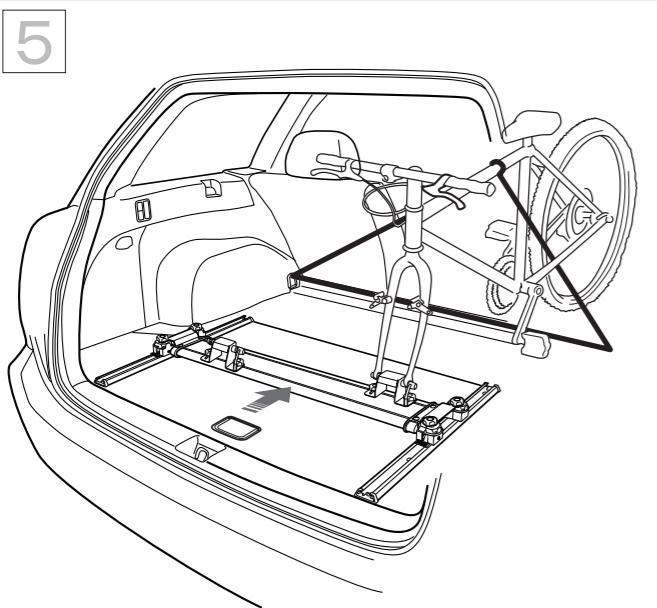
Be sure to fasten the Belt to the vehicle cargo hooks. It fastened the Belt to the hook of this Luggage Rail, the bicycle do not hold securely.
