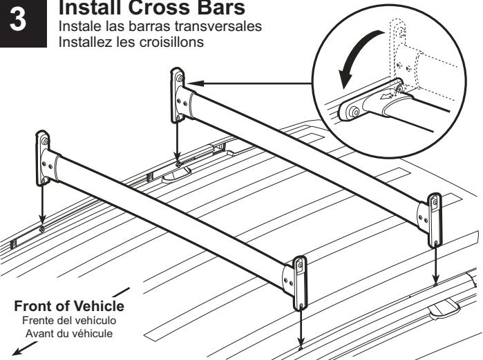
**CAUTION:** Failure to install crossbars in the proper orientation could lead to increased wind noise.
