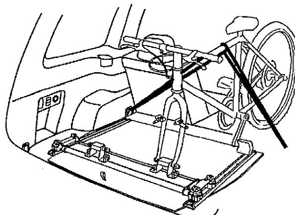
Be sure to fasten the Belt to the vehicle cargo hooks. It fastened the Belt to the hook of this Luggage Rail, the bicycle do not hold securely.
