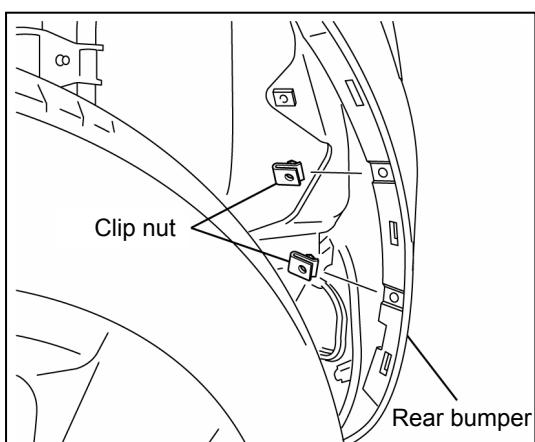
2. Align the rear bumper holes, and install the kit clip nuts (2).
