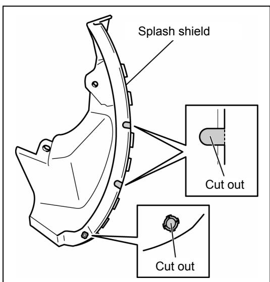
1. Cut off the splash shield shown in the figure using nipper (3 locations).
