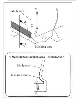
7. Apply a piece of masking tape at 8 mm away from the bottom end of the mudguard as shown in the left figure.
