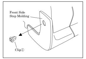
\*Assembled shape of the front side step molding\*
