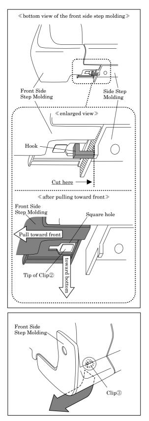
2. Cut out the hook of the side step molding with a nipper as shown in the enlarged view.
