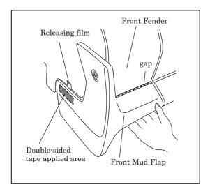
13. Lift up the front mud flap and make the gap between the front fender and the front mud flap constant from one end to another. While keeping the position, remove the releasing film and push the front mud flap toward the front fender in order to get good adhesion.
