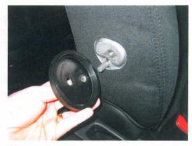
Place the cover-ring over the adapter bracket and mount the bracket over the axle-pin (so that it entry into the spline-tube)
