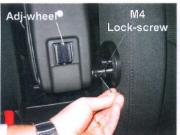
Secure the armrest on the adapter by tighten the M4 «lock-screw» (placed on the spline-tube). Then fold down the armrest and adjust the angle into a nice and relaxing position. Do not lean on the armrest while you adjust it!
