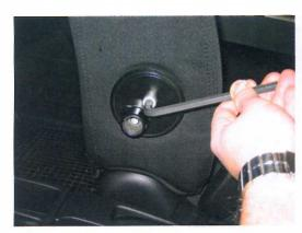
Secure the armrest by tighten the M10 insex-screw (use 8 mm insex-rod) and then cover the screw with the enclosed plastic-cap.
