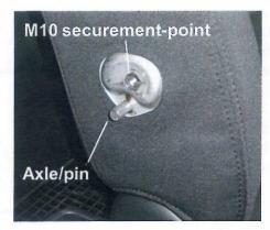
Remove the armrest and locate the two fastening points -the axle/pin and the M10 securement point.
