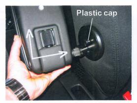
Mount the armrest into the spline-tube in a backfolded position and make sure the armrest stops in line with the seat.
