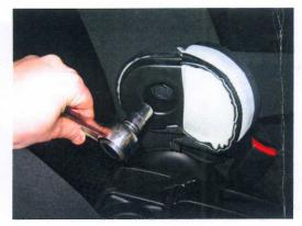
Use a 14 mm box-spanner to loose the centre screw on the armrest.
